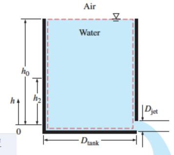
$$\int_{0}^{t} dt = -\frac{D_{\text{tank}}^{2}}{D_{\text{jet}}^{2} \sqrt{2g}} \int_{h_{0}}^{h_{2}} \frac{dh}{\sqrt{h}} \to t = \frac{\sqrt{h_{0}} - \sqrt{h_{2}}}{\sqrt{g/2}} \left(\frac{D_{\text{tank}}}{D_{\text{jet}}}\right)^{2}$$
