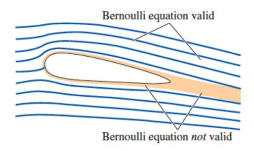
The sum of the kinetic, potential, and flow energies of a fluid particle is constant along a streamline, during steady flow, when compressibility and frictional effects are negligible.
