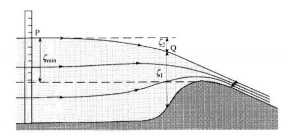
Calculate the flow rate as a function of  $\zeta_{min}$
