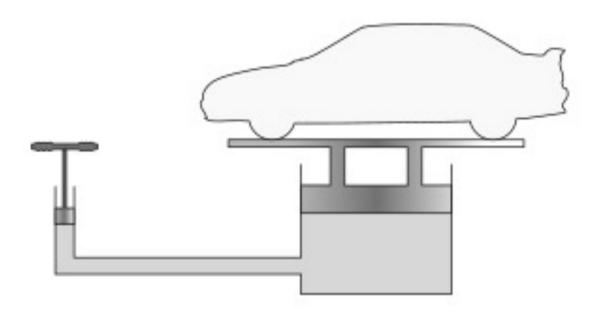
A change in pressure at any point in an enclosed fluid **at rest** is transmitted undiminished to all points in the fluid.
